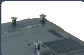
Step 1 attach height-adjustable standoffs to projector
