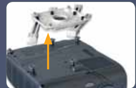
Lamp & filter access unlatch legs to disconnect interface from projector
