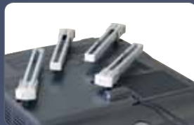
Step 2 latch legs onto standoffs
